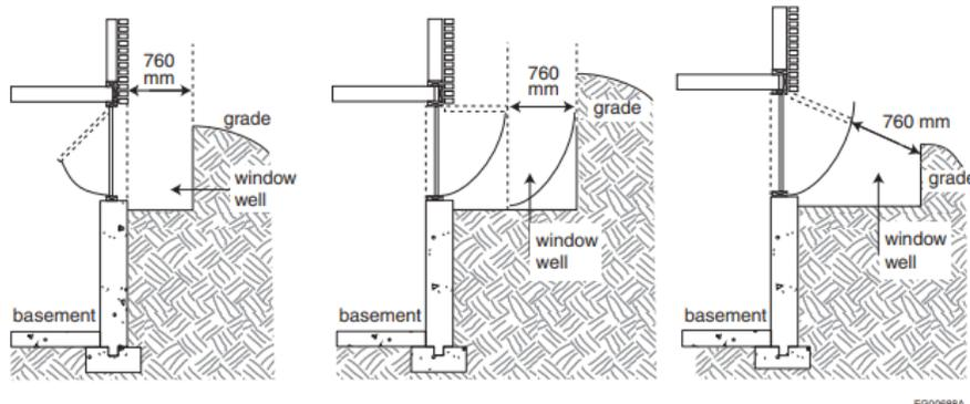
**BCBC 2018: Figure A-9.9.10.1.(3) Windows providing a means of escape that open into a window well.**
