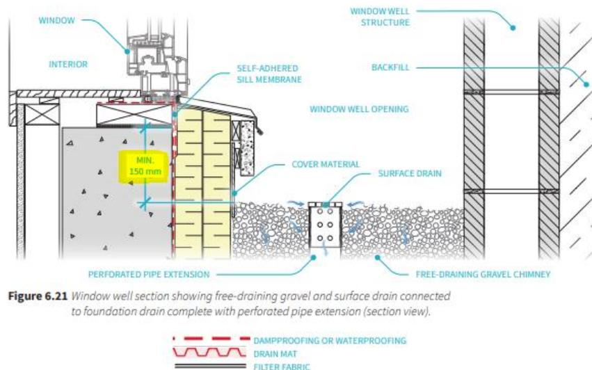
**Figure 6.21** Window well section showing free-draining gravel and surface drain connected to foundation drain complete with perforated pipe extension (section view).
