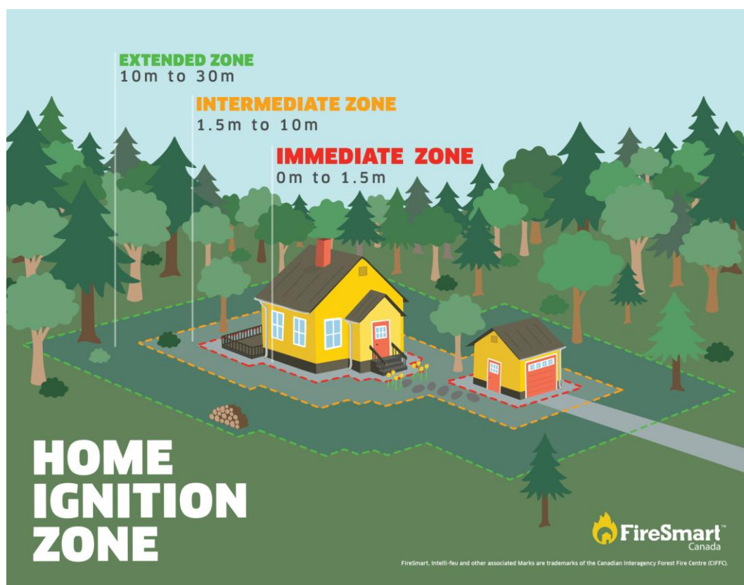
Figure 19. FireSmart Home Ignition Zone, which is comprised of four priority zones, as illustrated in the BC FireSmart Begins at Home Manual
