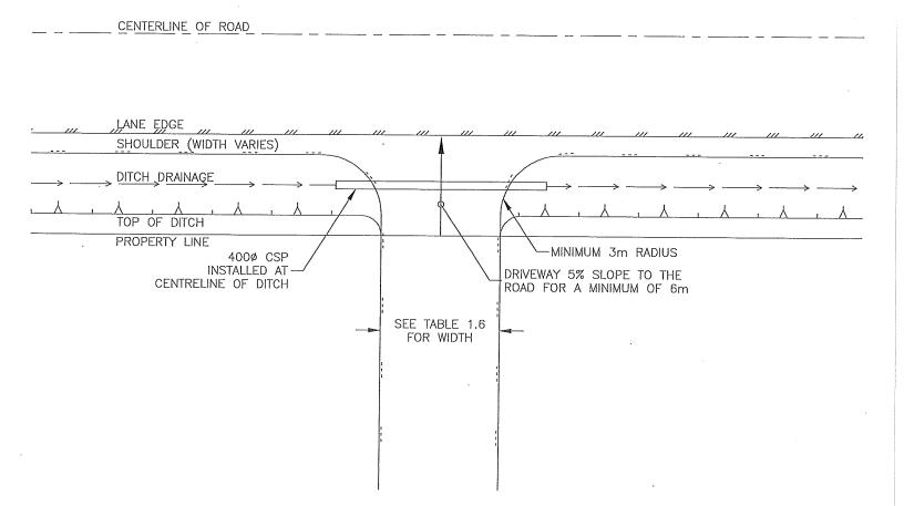
LOCATION, DESIGN AND CONSTRUCTION OF TYPICAL RESIDENTIAL DRIVEWAY AND CULVERT NOT TO SCALE
