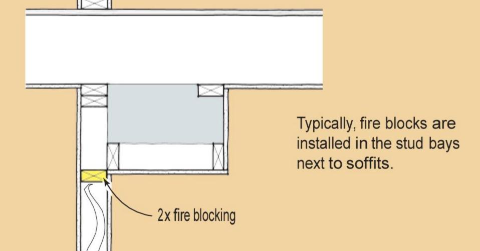
Installing a single piece of material across the face of the studs is often faster than using individual blocks. Approved materials include 2x lumber, <sup>3</sup>/<sub>4</sub>" structural sheathing, and 1/2" drywall.
