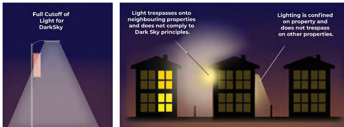
Figure 45: Examples of dark sky compliant lighting that protects visual spillage and glare on adjacent uses.
