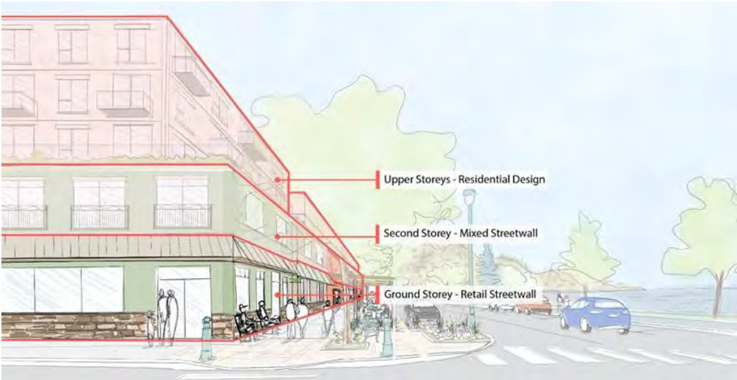
Figure 19: Building Design Treatment Hierarchy
