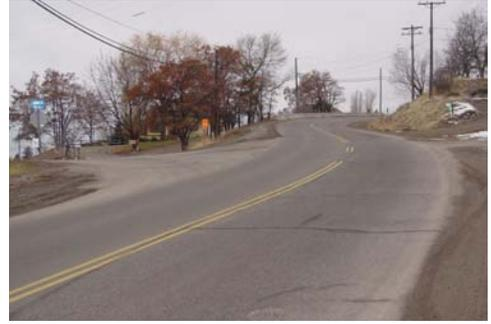
southbound right turn, and potentially reconstructing the driveways (and reducing the number) driveway on the north side of Princeton west of Lipsett. As well, the northbound approach lane should be at least 5 m wide at the intersection, so that left-turning vehicles do not impede right-turning vehicles.
